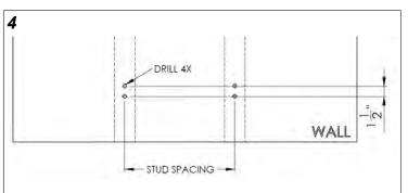
For Concrete Wall attachment: Use all 12 holes specified in Figure 5.
