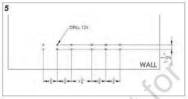
2. As required by the fastener manufacturer's recommendations, use the appropriate drill for the material to pre-drill holes on the wall in the specified positions.
