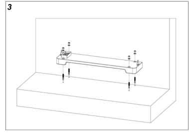
Tighten the bolts to manufacturer torque specifications. 6. Do a second check to make sure that the floor mount base is still level.
