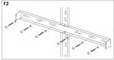
4. For each additional battery (up to three) in the stack, screw in the vertical spacer to the last horizontal retainer installed. Repeat steps 1 through 3 for each horizontal retainer, as shown in Figure 14 (for studs) or 15 (for concrete).
